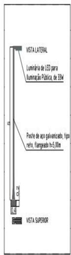
DETALHE POSTE DE AÇO GALVANIZADO SEMESCALA
